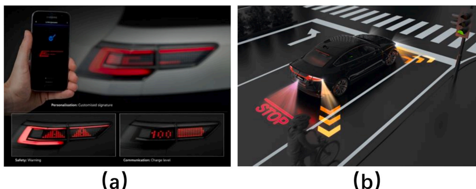
Fig. 1. (a): an example of matrix taillights; (b): an example of pixel-projected taillights (KURTULUS, 2021).
